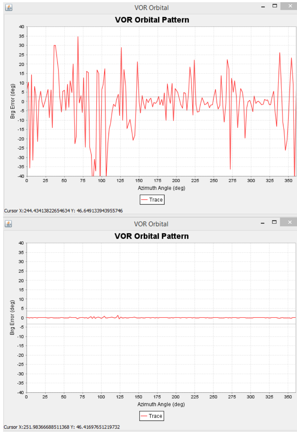
Figure 228: Results for Exercise 10 with all scatterer plates in place. Top is conventional VOR, bottom is doppler.
